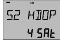
**4 SAT** indicates the number of satellites used min 3 and max 15. The GPS will internally track up to 12 satellites.
