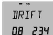
example, the boat is drifting on a bearing 234~ with the speed 0,8 knots.
