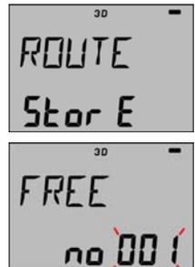
The first free ROUTE is no 001, press **SET** and give the route a name by using the **PLUS**, **MINUS** and **PAGE** buttons
