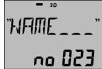
When the desired digit is flashing, enter the number with the **PLUS** or **MINUS** button and then move the cursor to the next digit. Press **SET** lock.
