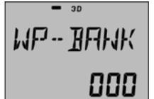
**This is a special function for transfer (import) of WP's FROM a NEXUS MASTER GPS Navigator instrument TO a NEXUS repeater instrument,**
